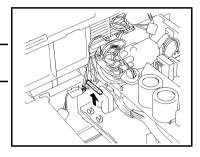
▲ Replace the Fuse of PU2.
